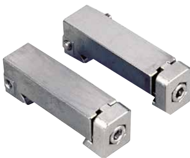
Reference stop, 3R-225.2 For positioning 3Ruler anywhere on the reference elements. The stops have adjusting screws for accurate alignment. • Tightening torque 7 Nm • Supplied in sets of 2 • Weight per set 0.6 kg
