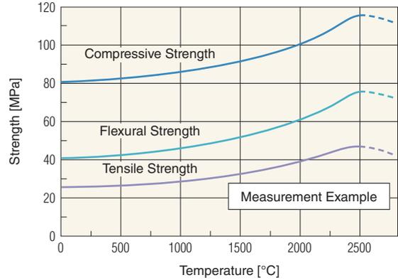
An unparalleled characteristic of graphite, which makes it indispensable in high temperature applications, is that as the temperature rises (up to 2,500°C), the strength also increases. Strength reaches levels approximately double those at room temperature.
