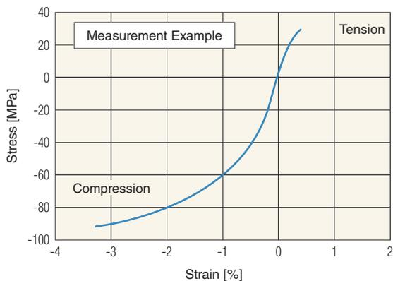
Graphite generally shows elastic-plastic deformation. The fracture behavior is different under tension and under compression, so caution must be exercised.
