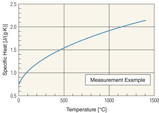
Due to the anisotropic nature of its crystals, the specific heat of graphite at room temperature stays at 1/3 of that of general solids. The specific heat value is essential in various thermodynamic functions. At high temperatures, specific heat values are similar regardless of the graphite grades.
