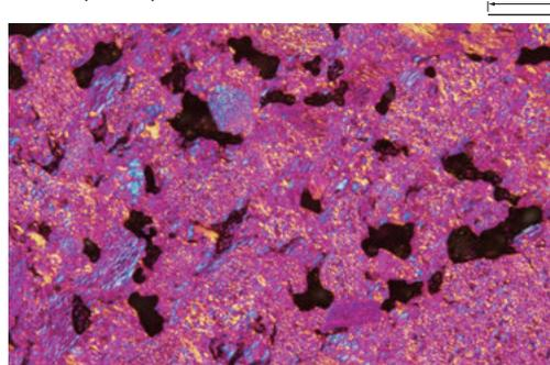
Isotropic high density graphite is different from conventional graphite in that it is isotropic and has a micro particle structure, creating a very strong and highly reliable material with a small variation. This isotropic graphite material resolves the problems associate with conventional anisotropic graphite.
