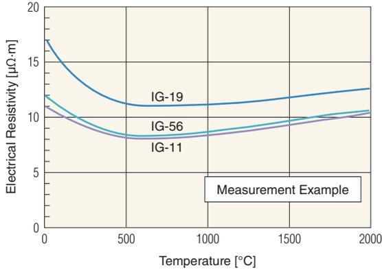
Since thermal characteristics differ from grade to grade, the coefficient of electrical resistivity must be carefully studied when selecting a grade for a heating element.
