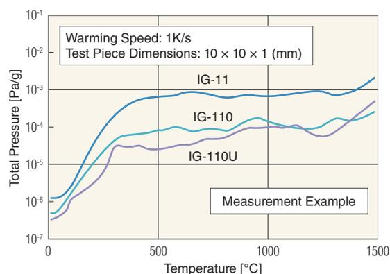
Graphite emits absorbed gas when in high temperatures. Some applications such as semi-conducting industries must use highly purified or ultra highly purified graphite, which emits less gas.
