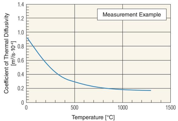
This chart shows that the higher the temperature rises, the faster the heat is transmitted. The thermal diffusivity of graphite is superior to other materials.
