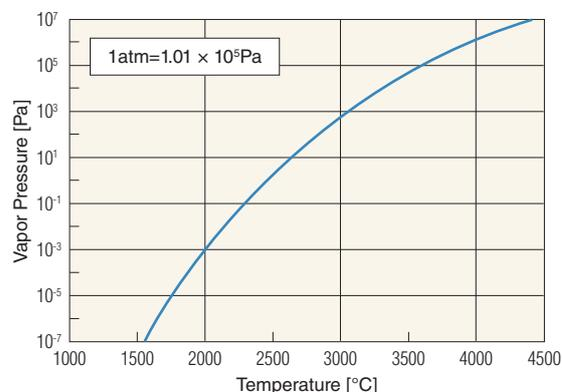
Graphite is an extremely stable material in temperatures under 2,200°C. However, the vapor pressure increases in higher temperatures and high vacuums, so caution must be exercised with regard to the accelerated wearing of graphite.
