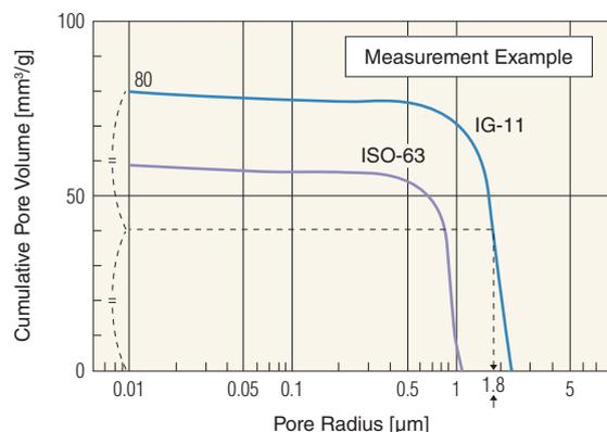
This shows the pore distribution through the mercury penetration method. The pore distribution has a close relationship with gas permeability and other unique properties of graphite. The halfway position of the cumulative pore volume indicates the average pore radius.
